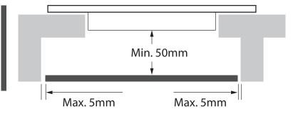
There are ventilation holes around outside of the hob. YOU MUST ensure these holes are not blocked by the worktop when you put the hob into position.
