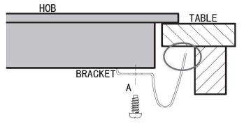
$\triangle$  Under any circumstances, the brackets cannot touch with the inner surfaces of the worktop after installation (see picture).
