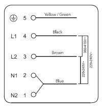
A If the total number of heating unit of the appliance you choose is not less than 4, the appliance can be connected directly to the mains by single-phase electric connection, as shown below.
